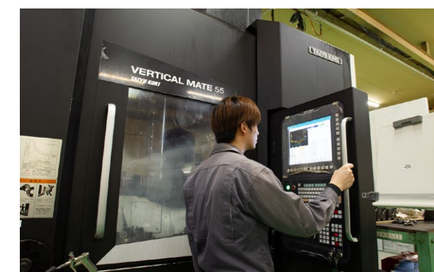
▲立形複合研削盤 Vertical Mate 55
